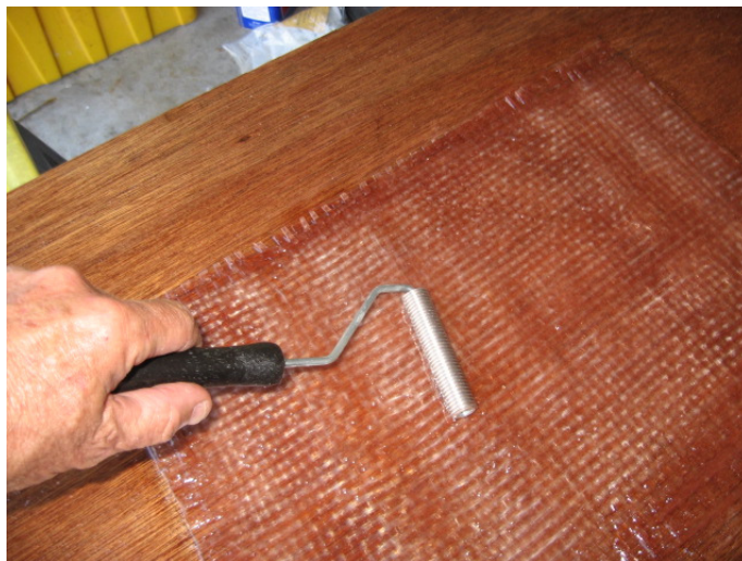
Figure 4 A laminating roller removes trapped bubbles
