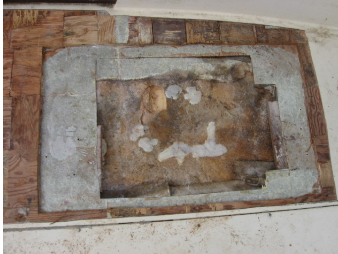
Figure 1 Cut out showing ledge and underdeck
