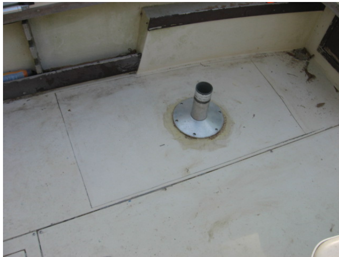
Figure 7 The finished repair with pedestal base installed
